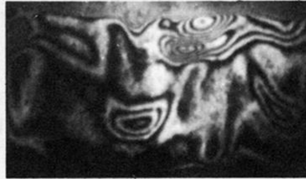
FIGURE 7. Laboratory Bénard-flow, taken from a film, with the permission of P. Bergé and M. Dubois, C.E.N. Saclay, Gif-sur-Yvette, France.
