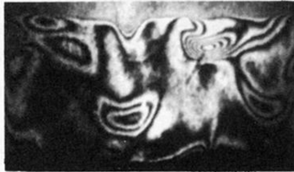
FIGURE 7. Laboratory Bénard-flow, taken from a film, with the permission of P. Bergé and M. Dubois, C.E.N. Saclay, Gif-sur-Yvette, France.
